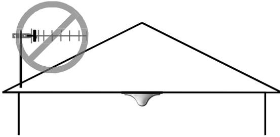
If light A is red, the amplifier has shut down due to oscillation. Verify that the outside Yagi antenna is pointed away from the inside antenna and not across the roof of the building. If need be, redirect the Yagi antenna so that it is pointing away from the inside antenna. Then, reset the amplifier by disconnecting and reconnecting the power supply. See “Cell Phone Overload Protection” on page 11.
