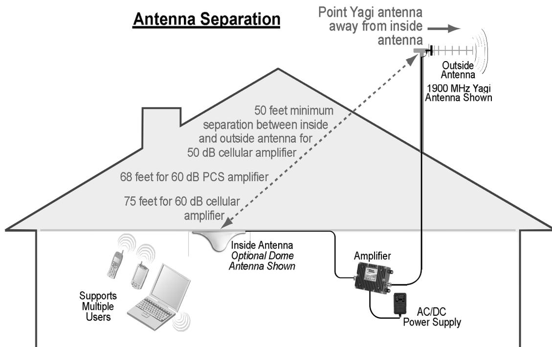
Connect the outside antenna to the amplifier with 9913 or equivalent coax cable (available from Wilson Electronics). Place the inside antenna in the center of the area needing the amplified signal. It is important to have at least 50 feet of separation between the inside and outside antennas for the 50 dB amplifiers, 68 feet of separation distance for the 60 dB PCS amplifiers, and at least 75 feet of separation distance for the 60 dB cellular amplifiers.
