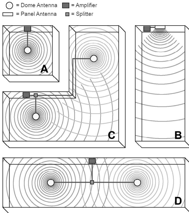
Connect the coax cable from the amplifier to the inside antenna. For distances of 20 feet or more, use 9913 coax cable or equivalent to prevent significant signal loss.
