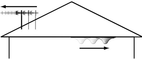
If light A is still red, increase the separation distance between the inside and outside antennas. Then, reset the amplifier by disconnecting and reconnecting the power supply. If light A is now green, there is sufficient antenna separation. If not, repeat this procedure.
